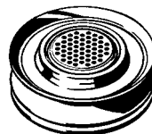
The Dosing Capsule inserted into the Filling Chamber Reducer
