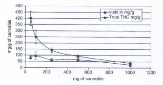
Figure 4. Total yield and total THC content of the condensates when different sample sizes were vaporised at 230°C.
