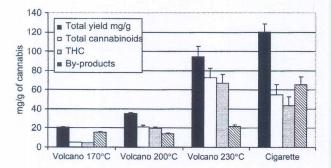
**Figure 2.** Experiment conducted in order to compare cannabis cigarette smoke with the vapor produced at different temperatures. For all the samples the total yield (dried condensate), total cannabinoids, THC, and total by-products are given in mg/g of cannabis plant material.
